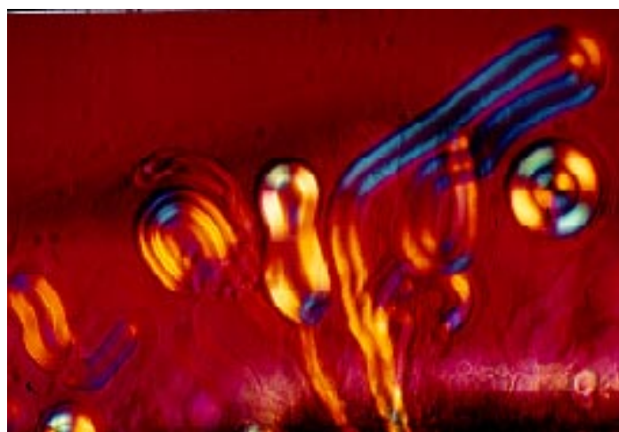
Fig. 90 PLM picture of dried cream layer (1 h, 33000 g) of autoclaved 20% w/w model emulsion after addition of double-distilled water ( 4444 = 45 \mu\text{m} )
