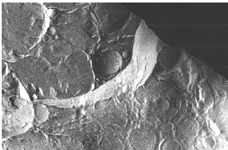
Fig. 86 FF-TEM micrograph of the centrifuged cream layer (1 h, 33000 g) of non-autoclaved 20% w/w model emulsion with 1.2% w/w Lipoid E80 ® showing densely packed droplets (4444 = 260 nm)
